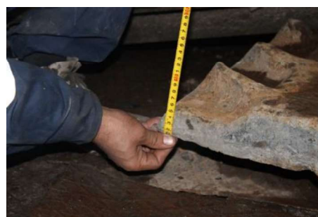
Fig. 5. Process of measuring worn liners and dismantling of worn liner plates (characteristic wear profile)
