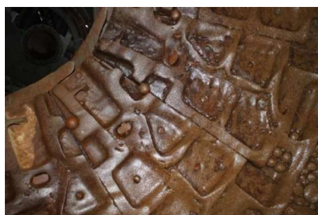
Fig. 5. Process of measuring worn liners and dismantling of worn liner plates (characteristic wear profile)
