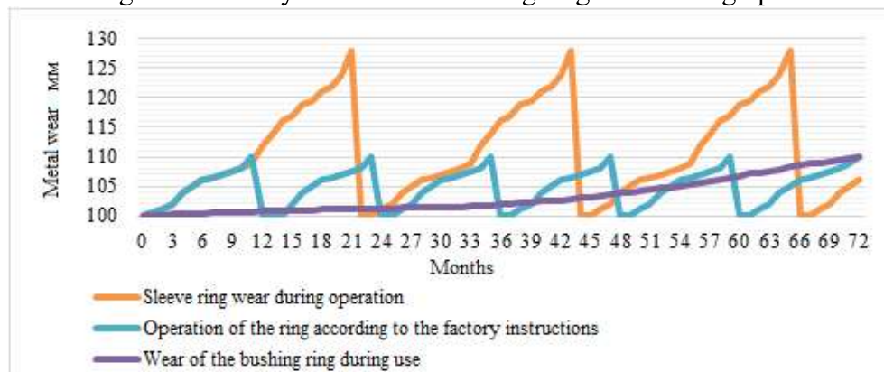
Figure 10. Graph of wear of the metal of the bucket ring depending on time
