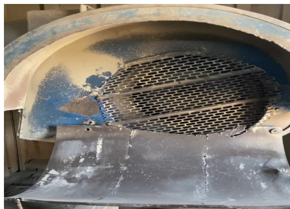
(b) filter cleaning device in the factory
